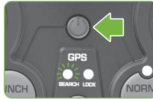
Turn on controller. Once paired with the drone, RED SEARCH LED will blink while acquiring GPS signal.
