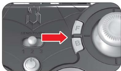
**IF DRONE DRIFTS FORWARD:** Press "F" button several times until drone stops drifting forward.
