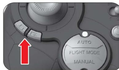
**IF DRONE SPINS COUNTER-CLOCKWISE (VIEWED FROM ABOVE):** Press the "R" button several times until drone stops spinning.
