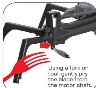
Using a fork or tool, gently pry the blade from the motor shaft.
