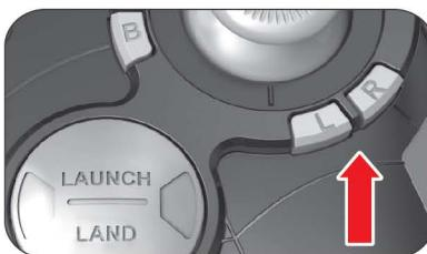
**IF DRONE DRIFTS LEFT:** Press "L" button several times until drone stops drifting left.
