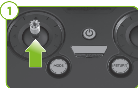
Raise the throttle stick to arm the frame. The motors will spin, indicating the frame is armed. Increase throttle to lift off of the ground.
