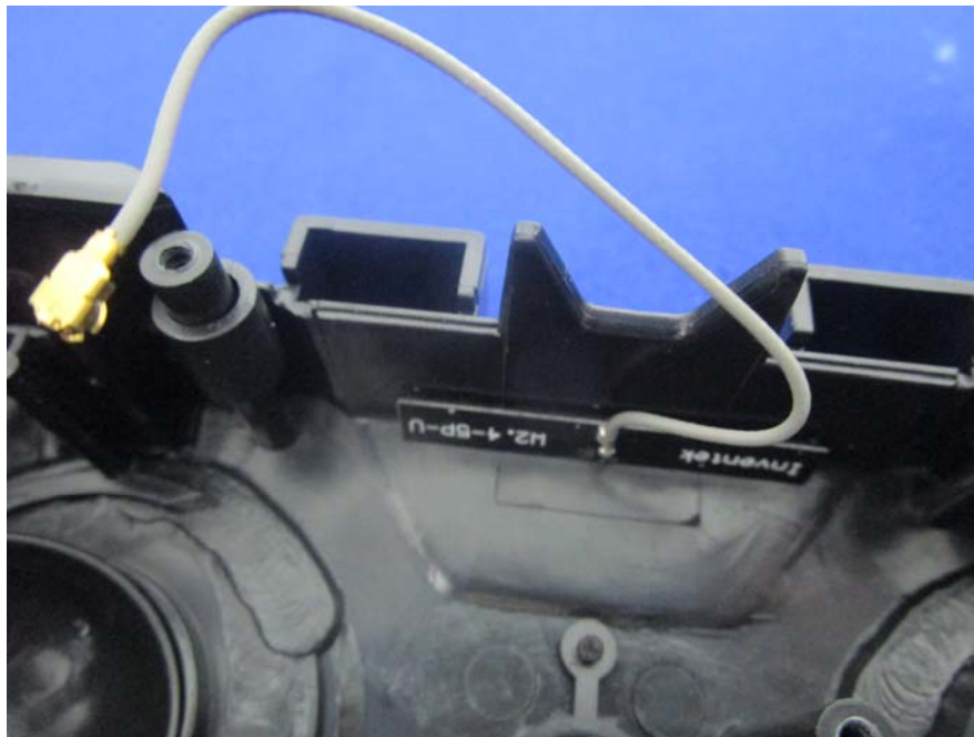
EUT – RF Antenna View
