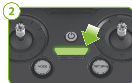
When enough satellites are locked on, the GPS LOCK will illuminate a solid GREEN. The frame is now ready to fly in GPS mode.
