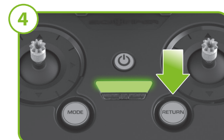
When flying in GPS mode, press the RETURN button to RETURN HOME. The frame will fly back to the home location and land. RETURN HOME will ONLY work if GPS LOCK is active.
