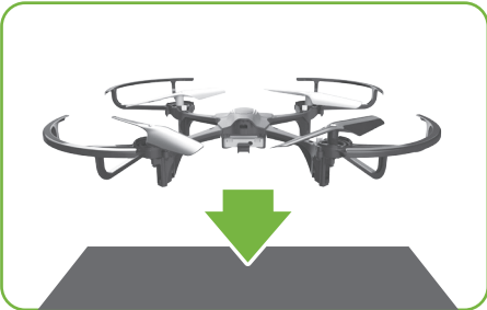
Place the drone on level surface for calibration.
