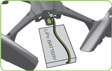
Insert fully charged LiPo battery into the underside of the drone, then connect the battery to back of the drone. [See reverse.]
