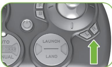
**IF THE DRONE DRIFTS LEFT:** Press "R" button several times until the drone stops drifting left.
