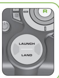
Press **LAUNCH** to automatically launch a few feet off the ground.
