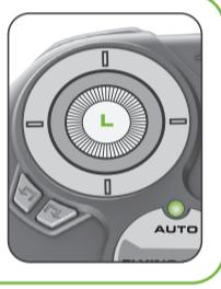
Move **LEFT (Throttle)** thumbstick up or down to make drone fly higher or lower and left or right to rotate.
