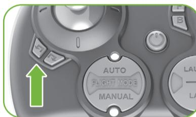
**IF THE DRONE SPINS COUNTER-CLOCKWISE (VIEWED FROM ABOVE):** Press the L button several times until the drone stops spinning.
