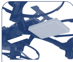
Pull battery out
