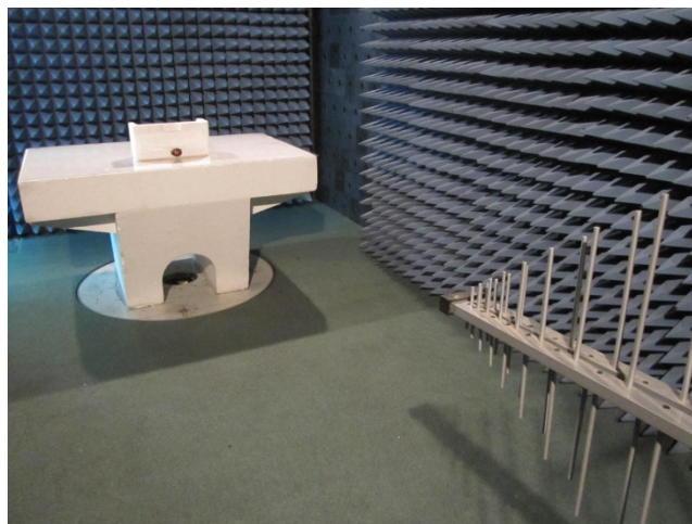
Photograph 8.1.1 Setup for spurious emission field strength measurements from 30 to 1000 MHz
