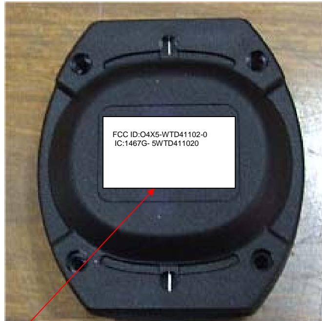
Label with **FCC ID:O4X5-WTD41102-0** and **IC:1467G-5WTD411020** is located at the rear side panel of the Wrist tag. The statement according to FCC part 15 §15.19(a)(3) is placed in User's Guide, page 4 (Application exhibit [User\\_manual\\_26148](#)).
