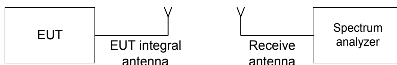
Figure 7.1.1 Setup for transmitter shut down test
