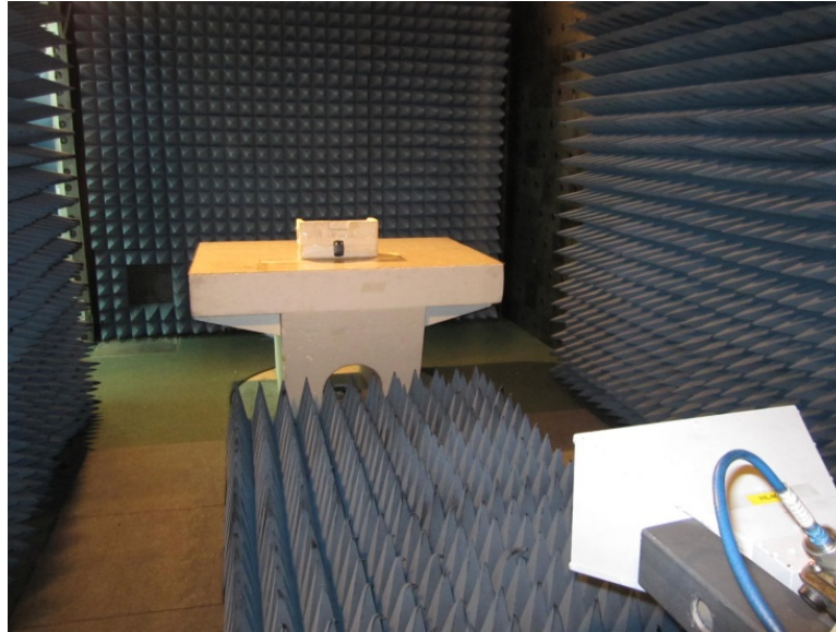
Photograph 8.1.3 Setup for final radiated emission measurements, EUT close view
