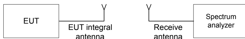
Figure 7.1.1 Setup for transmitter shut down test
