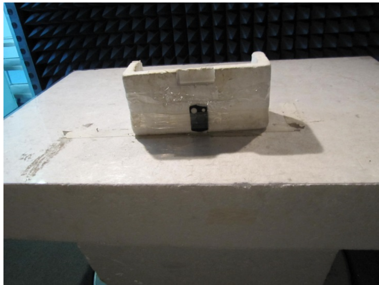
Photograph 8.1.3 Setup for final radiated emission measurements, EUT close view
