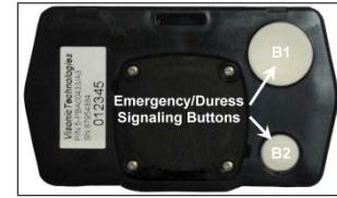
When the buttons are released, B1=0 and B2=0. Another RF message is transmitted until it receives the Ack message or tries five more times. In the steady state (no button press / button release) B1=0 and B2=0.
