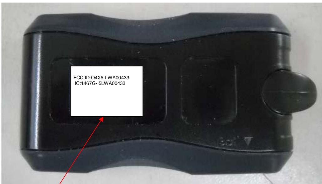
Label with **FCC ID:O4X5-LWA00433** and **IC:1467G-5LWA00433** is located at the rear side panel of the Lone Worker active RFID tag. The statement according to FCC part 15 §15.19(a)(3) is placed in User's Manual, page 4 (Application exhibit 5-LWA\_UserMan).
