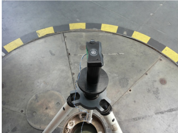
Photograph 6.4.2 EUT in Y-axis orthogonal position
