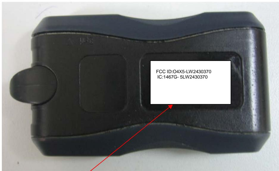
Label with **FCC ID:O4X5-LW2430370** and **IC:1467G-5LW2430370** is located at the rear side panel of the tag. The statement according to FCC part 15 §15.19(a)(3) is placed in User's Guide, page 6 (Application exhibit User\_manual\_27065).
