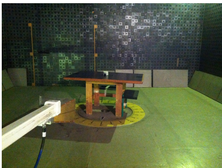
Photograph 8.1.2 Setup for radiated emission measurements
