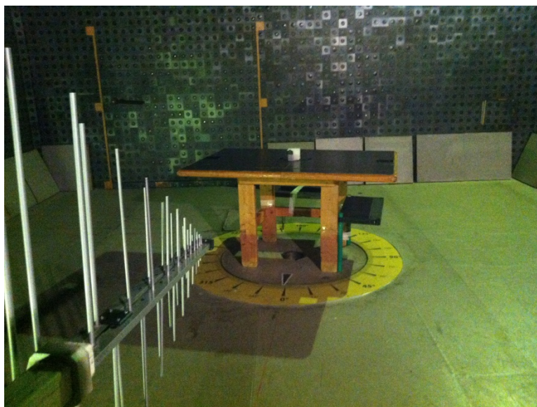
Photograph 8.1.1 Setup for radiated emission measurements
