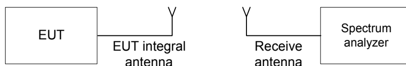
Figure 7.1.1 Setup for transmitter shut down test
