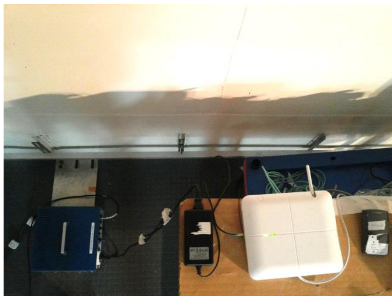
Photograph 8.1.1 Setup for conducted emission measurements
