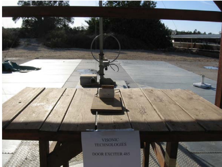
Figure 2. Radiated Emission Test
