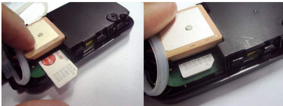
Picture 15: SIM Card Insertion > Positioning
