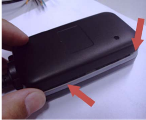
Picture 16: SIM Card Insertion > Rubber gasket
