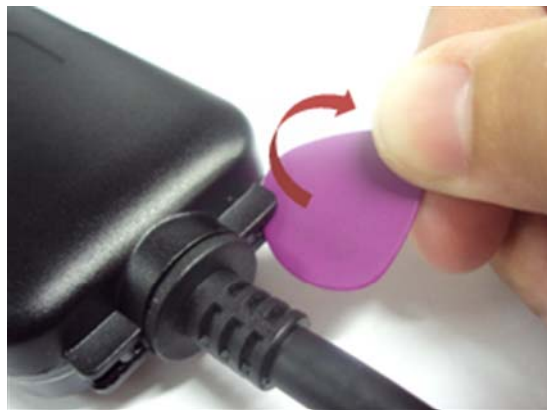
Picture 12: SIM Card Insertion > Detaching top cover
