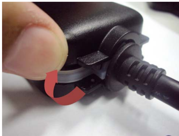
Picture 13: SIM Card Insertion > Detaching bottom cover
