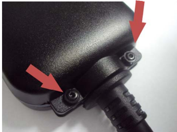
Picture 11: SIM Card Insertion > Removing screws
