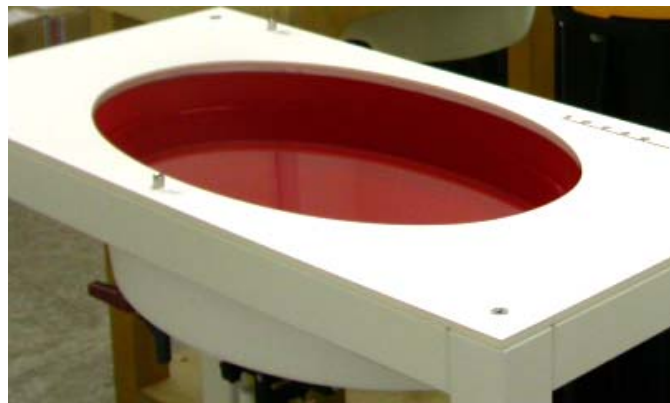
Fig. 8 SAM Twin Phantom and ELI4 Phantom
