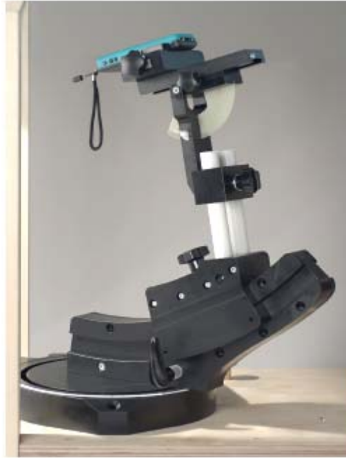
Fig. 9 Device holder supplied by SPEAG
