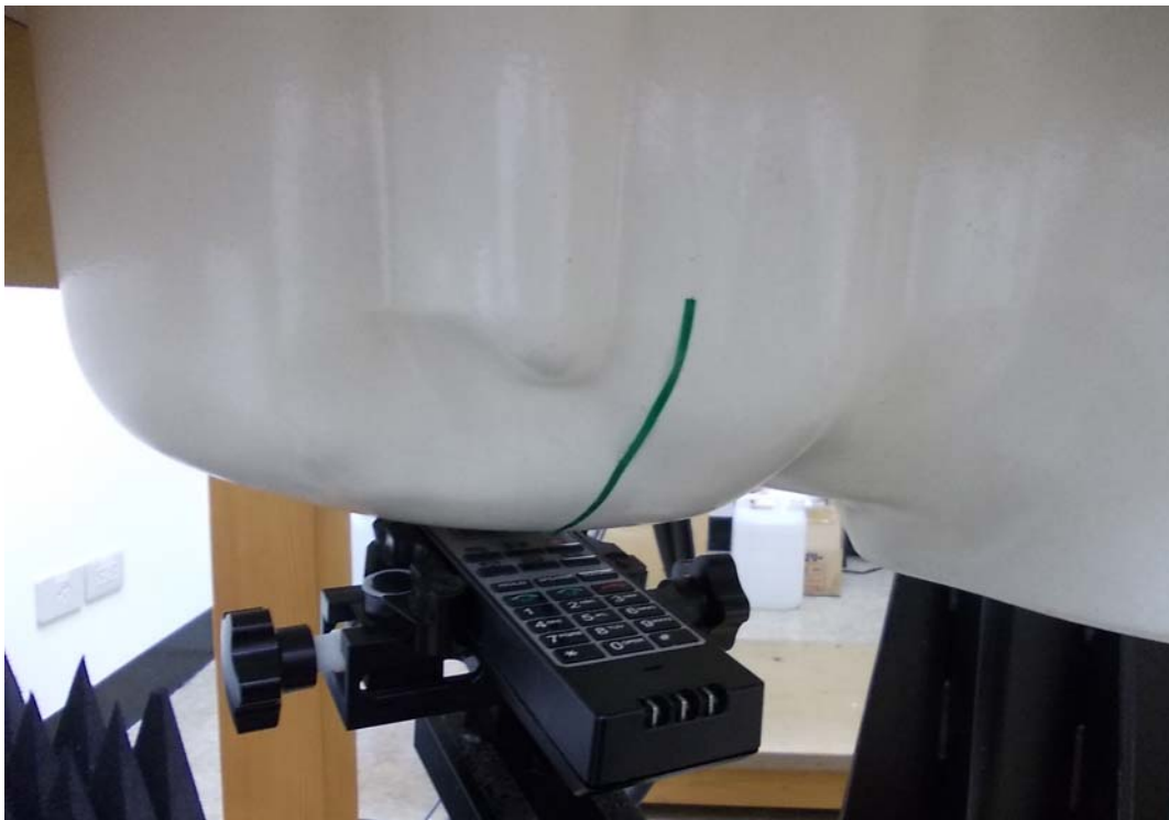
Measurement Position of Right-Tilt (RT) with Handset
