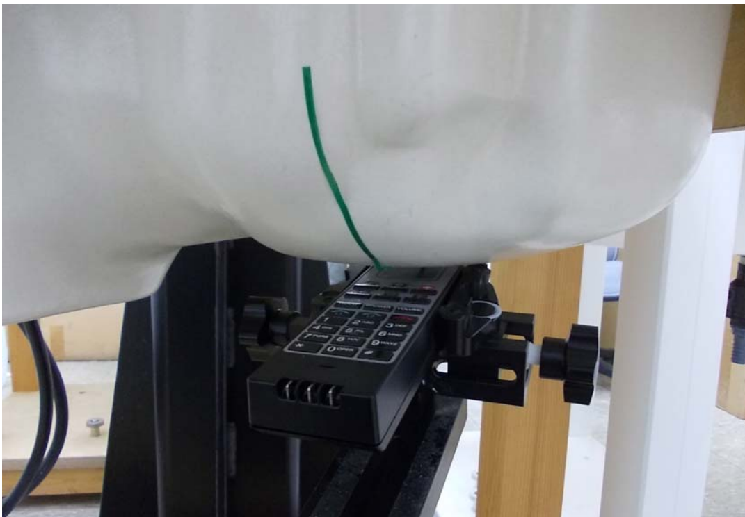
Measurement Position of Left-Tilt (LT) with Handset
