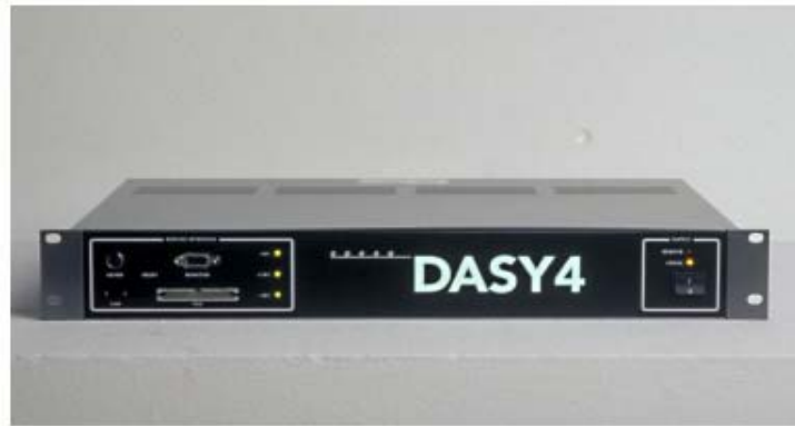
Fig. 6 DASY4 Measurement Server
