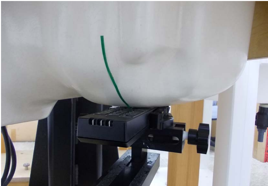
Measurement Position of Left-Cheek (LC) with Handset
