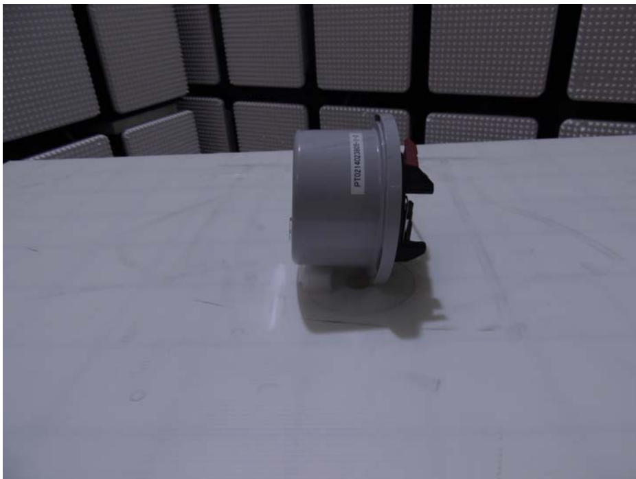
Photograph 7: Set-up for Radiated Emission, EUT Configuration Y-Axis
