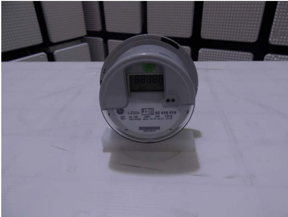
Photograph 6: Set-up for Radiated Emission, EUT Configuration X-Axis
