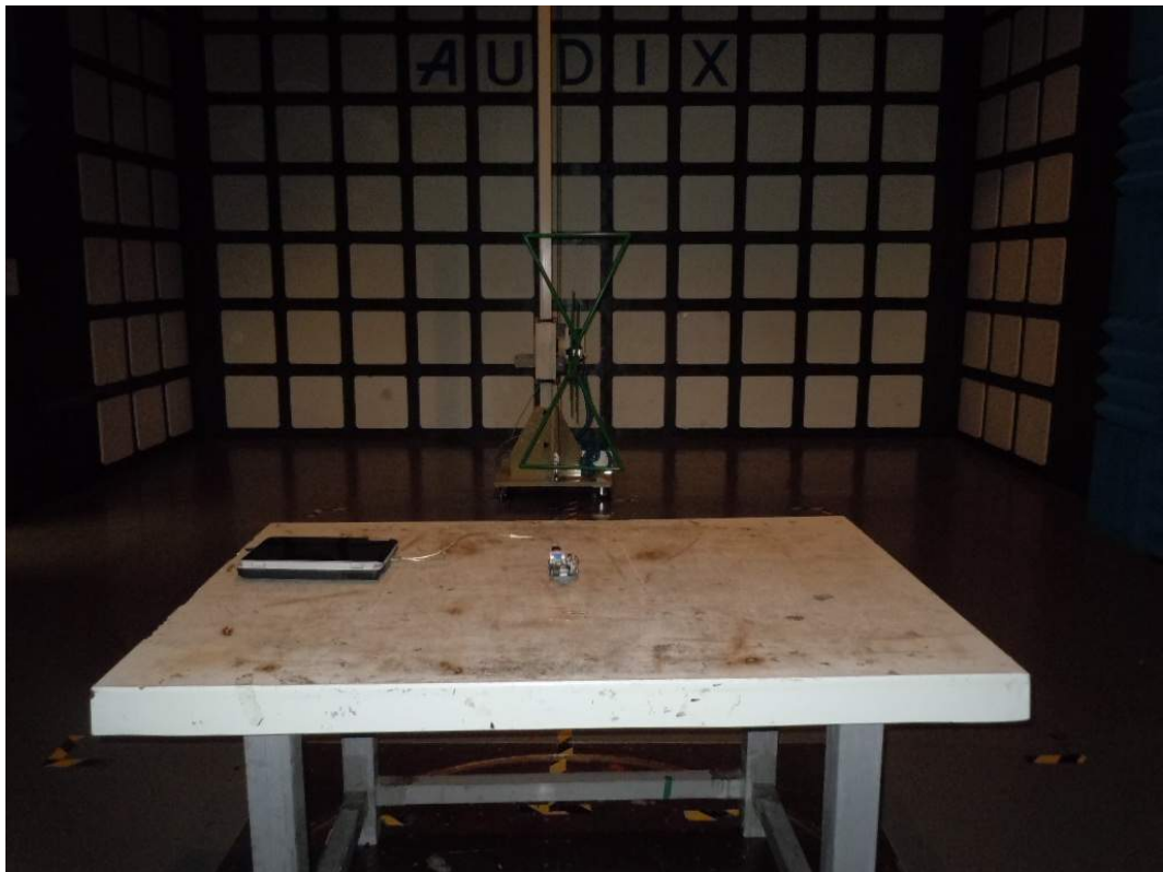
FRONT VIEW OF RADIATED EMISSION TEST (PCB ANTENNA BELOW 1GHz)
