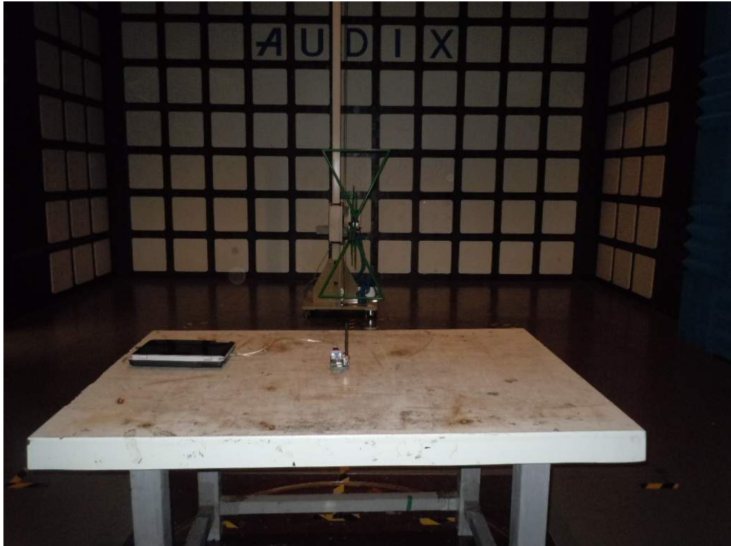
FRONT VIEW OF RADIATED EMISSION TEST (SMA ANTENNA BELOW 1GHz)
