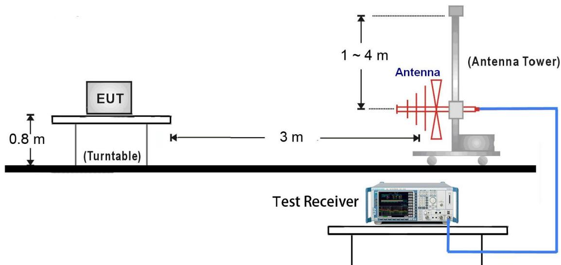
1GHz ~ 25GHz Test Setup:
