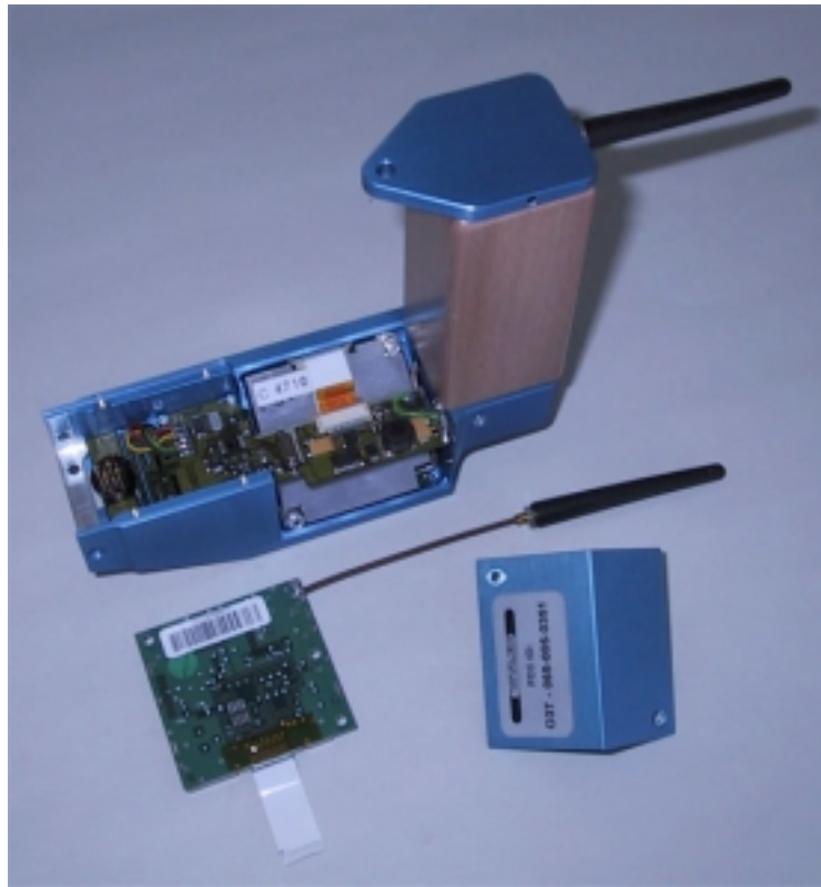
Handle of the Instrument MINILEVEL NT with integrated Radio Transmission Module dismantled (Antenna with Module and Cover)
