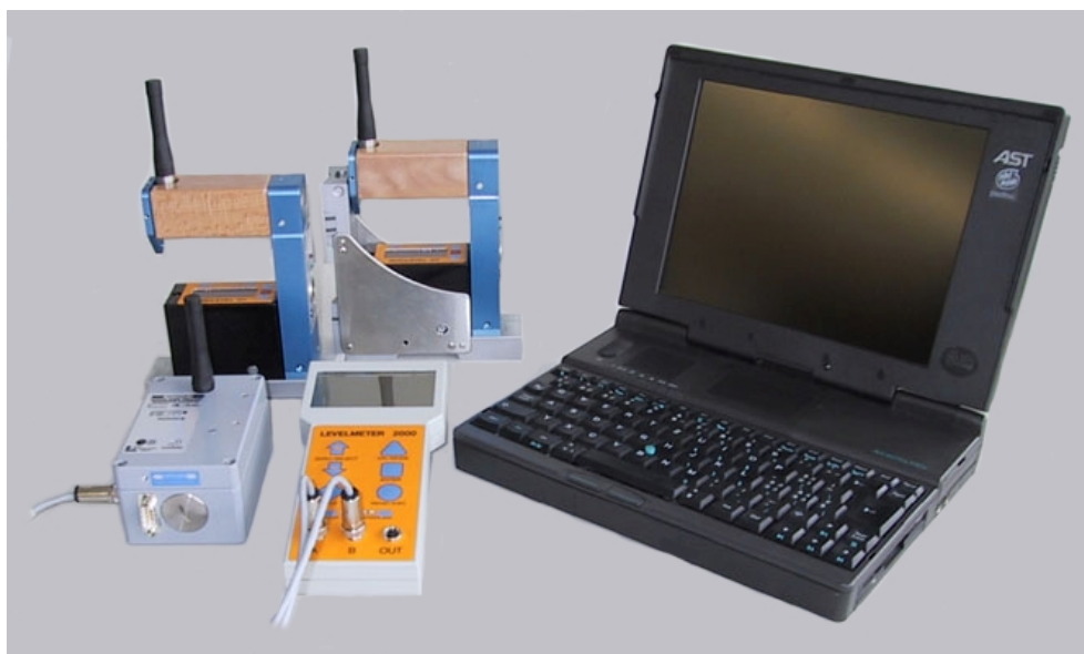
2 MINILEVEL NT with LEVELMETER 2000 and radio transmission module as an engineer set
