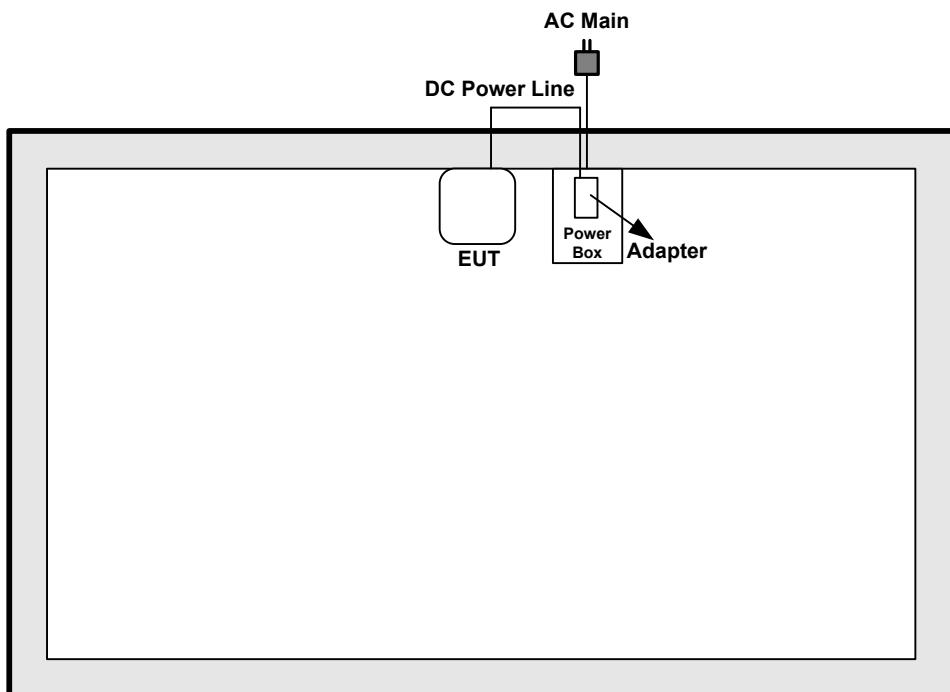
**Test Setup Diagram - Radiated Test (Above 1GHz)**
