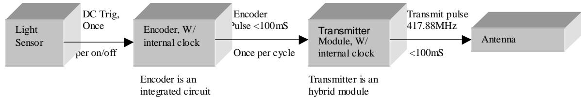
All clock signals are integrated within commercial purchased integrated circuits and hybrid modules.
