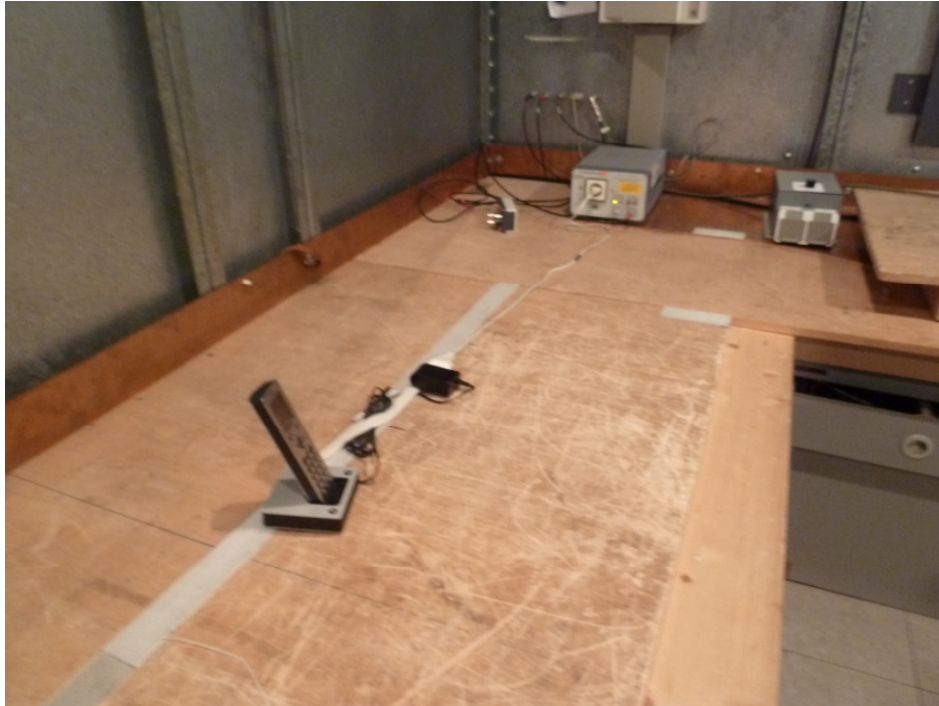
Photo 1: Power Line Conducted Emission Test
