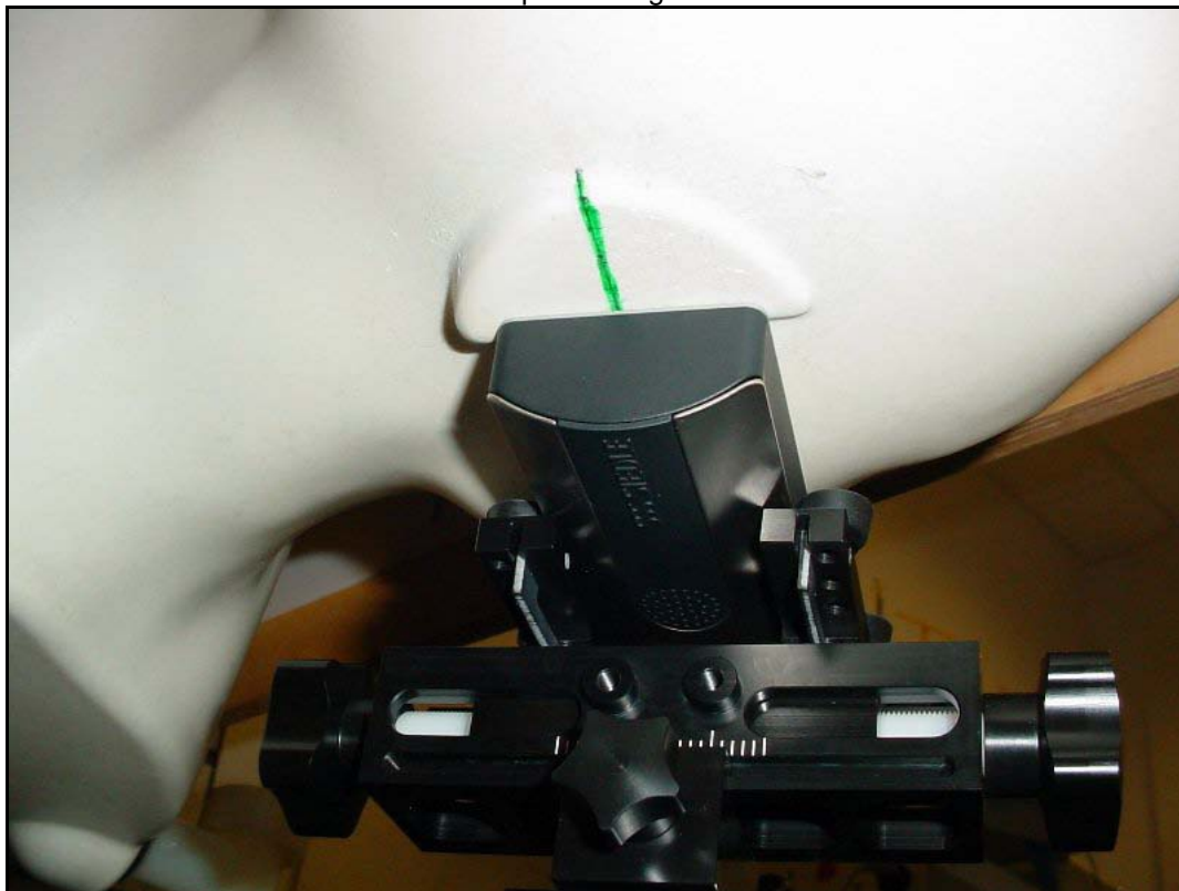
Photo 14: Test position right hand tilted 15°
