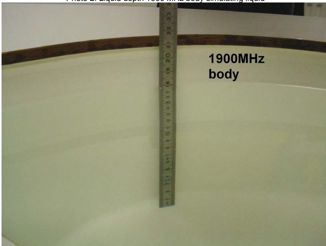
Photo 2: Liquid depth 1900 MHz body simulating liquid
