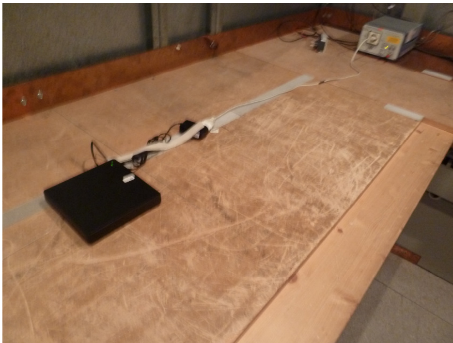
Photo 2: Power Line Conducted Emission Test
