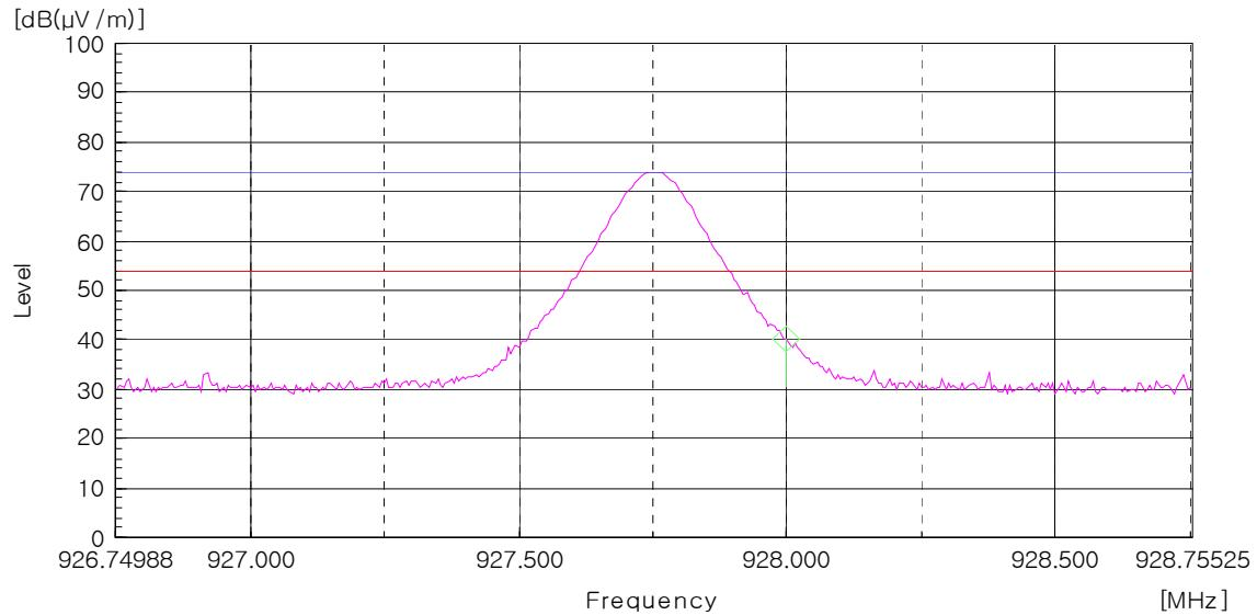
AV Detector: RBW: 1MHz, VBW: 10 Hz (926.749 MHz - 928.755 MHz), Worst case (High, Vertical)
