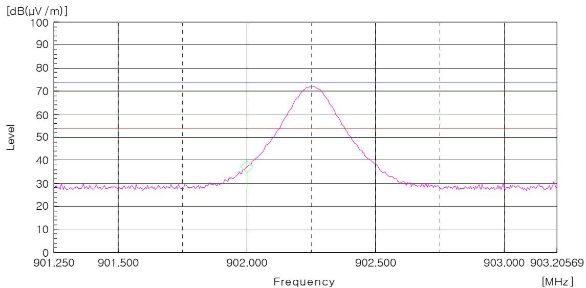
AV Detector: RBW: 1 MHz, VBW: 10 Hz (901.250 MHz - 903.205 MHz), Worst case (Low, Vertical)
