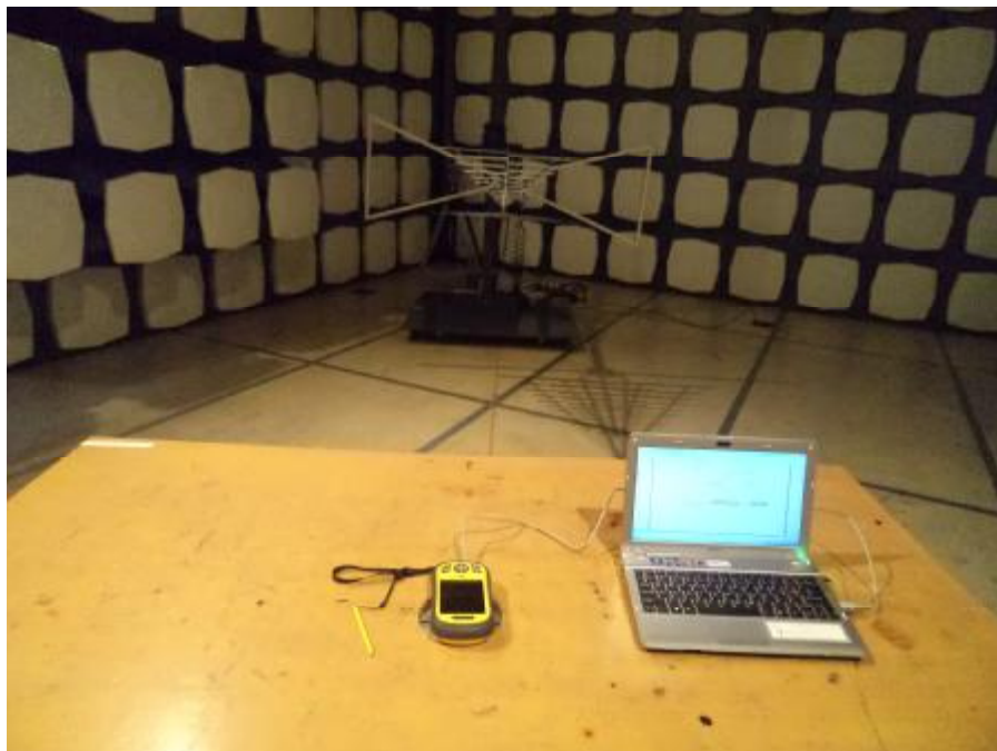
FCC RADIATED EMISSION TEST SETUP-Reading
