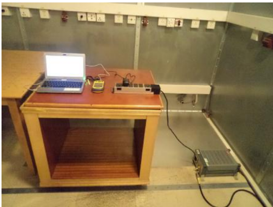
FCC CONDUCTED EMISSION TEST SETUP-Reading
