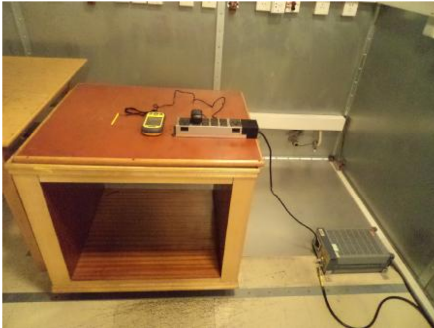
FCC CONDUCTED EMISSION TEST SETUP-Charging
