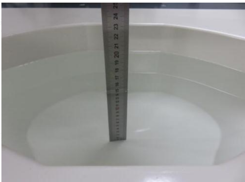
Photograph of the depth in the Body Phantom (2600MHz, 15.5cm depth)
