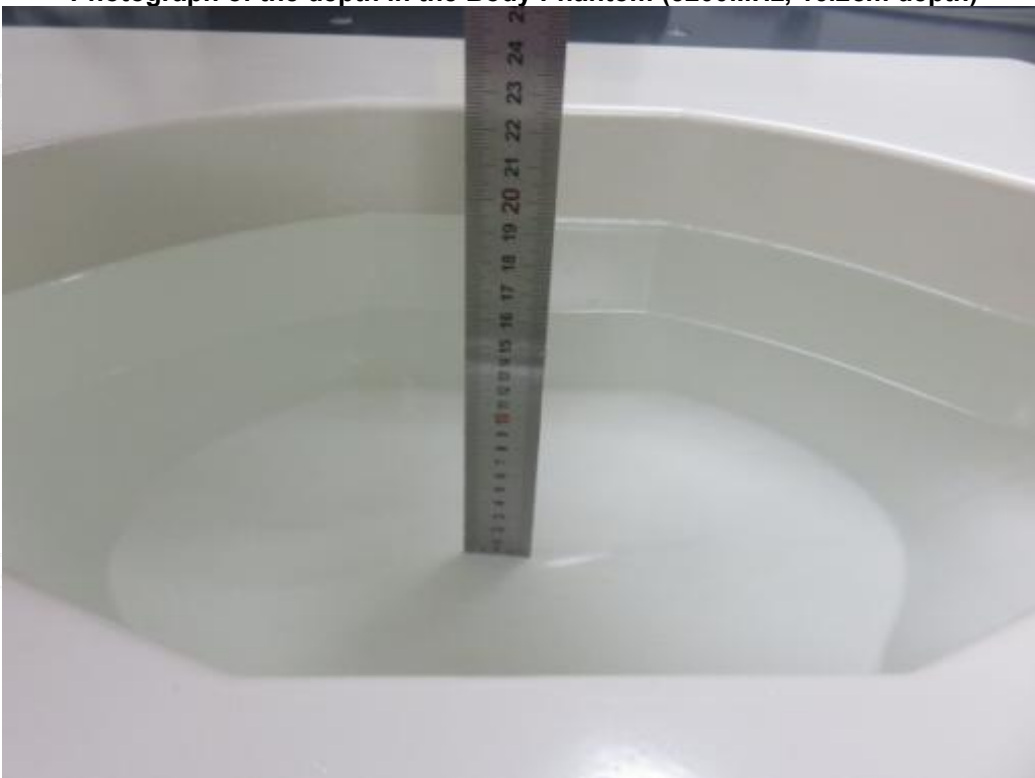
Photograph of the depth in the Body Phantom (5400MHz, 16.1cm depth)
