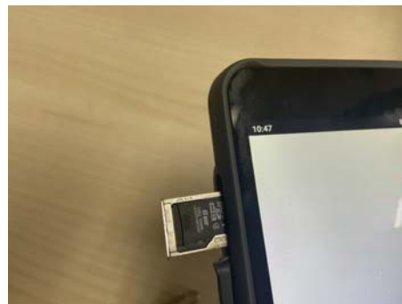
Figure 1-4-8 Installation of Micro SD card
