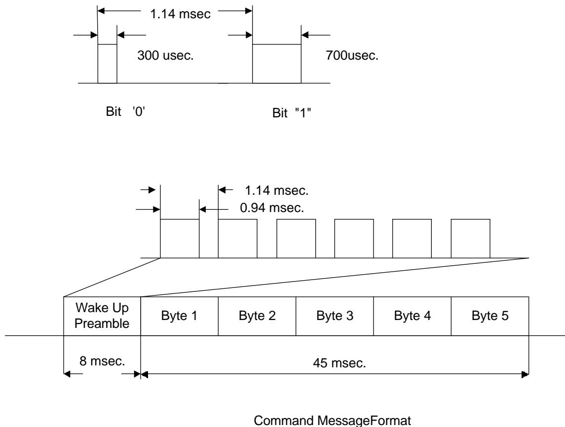
**Figure 4. Transmitted Data Format**
