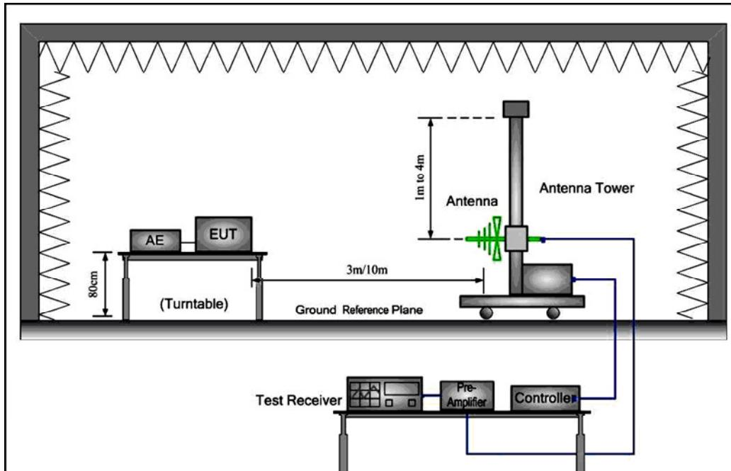
**1) Fundamental emission:****Antenna polarization: Vertical:**
