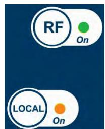
**i** The transmitter is working properly when: the CPU LED blinks, and both the RF LED and the interlock LED are green
