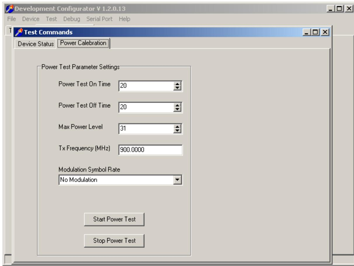
In this menu, specific power tests can be performed. The On/Off time can be chosen, the maximum power level and also the wanted frequency to transmit on. Also a modulation symbol rate can be chosen. With the [Start Power Test] and [Stop Power Test] the power amplifier is turned on and off.
