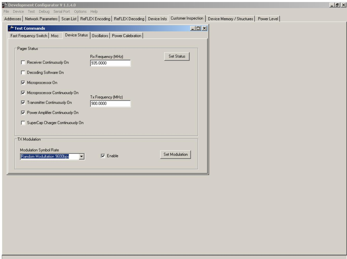
In this menu, power is set according to the level 0 (norml operation power level). The frequency can be chosen in the frequency field. Also a modulation symbol rate can be chosen. With the set status the power in set continuously on.
