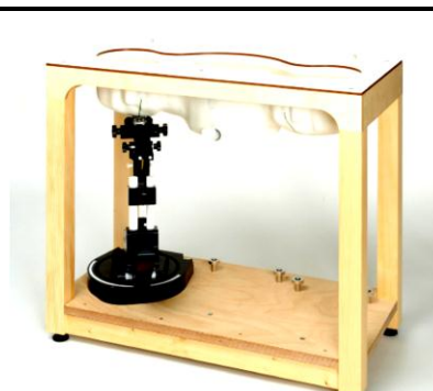
Fig 5.9 Photo of SAM Phantom
