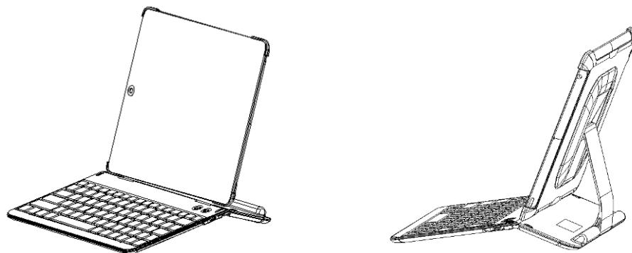
Remark: To get good stabilization, please kindly note the angle of machine and table is not more then 90 degree when adjust the Link
