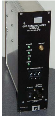
Figure 2-1 GPS-1 Synchronizer Module
