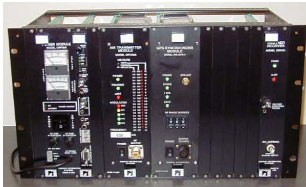
Figure 2-2 BlackMax Rack with GPS-1 and DRTXM3 Transmitter Installed
