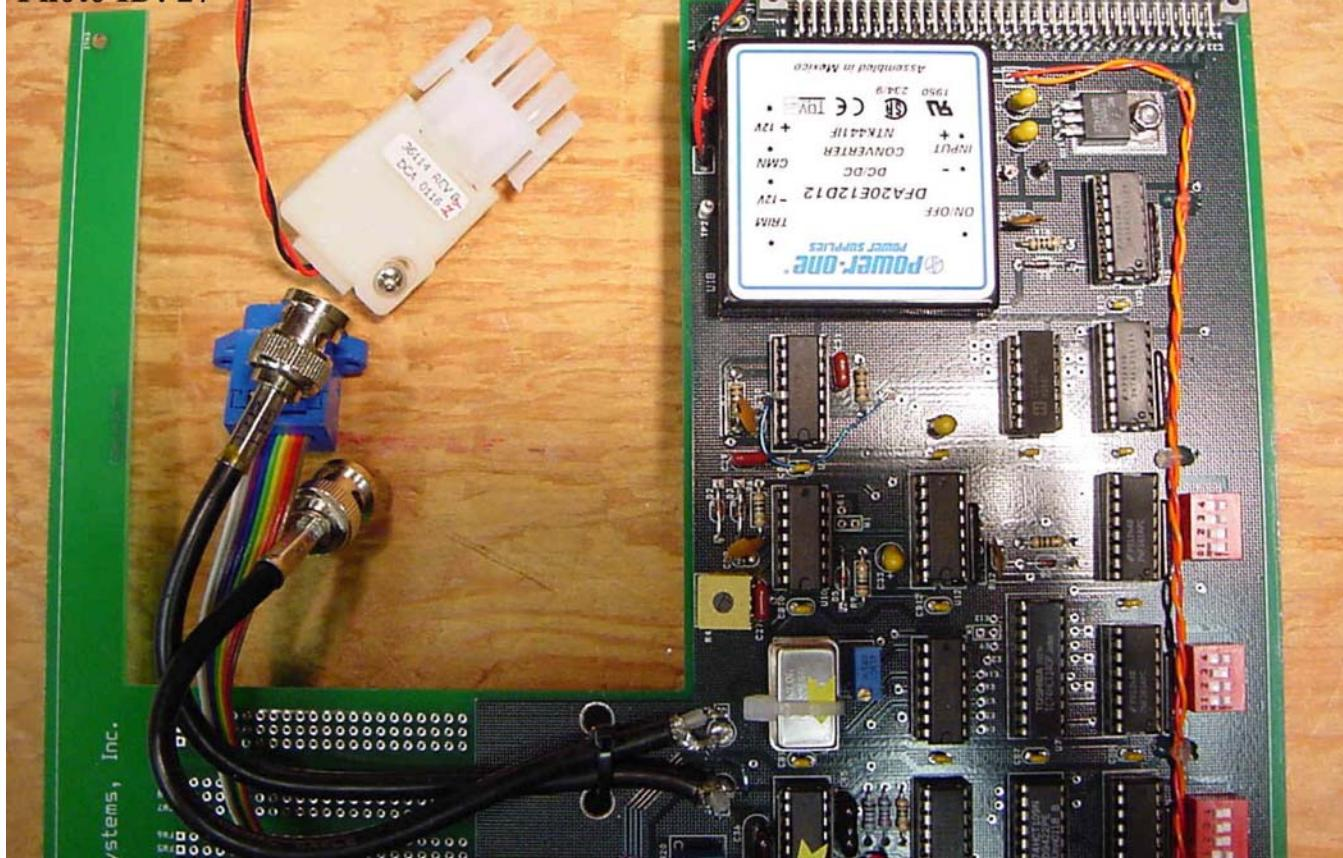
Back Half (component side) of the GPS-1 Circuit Board
