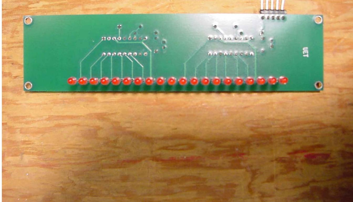
Solder/LED side of the DRTXM3 circuit board
