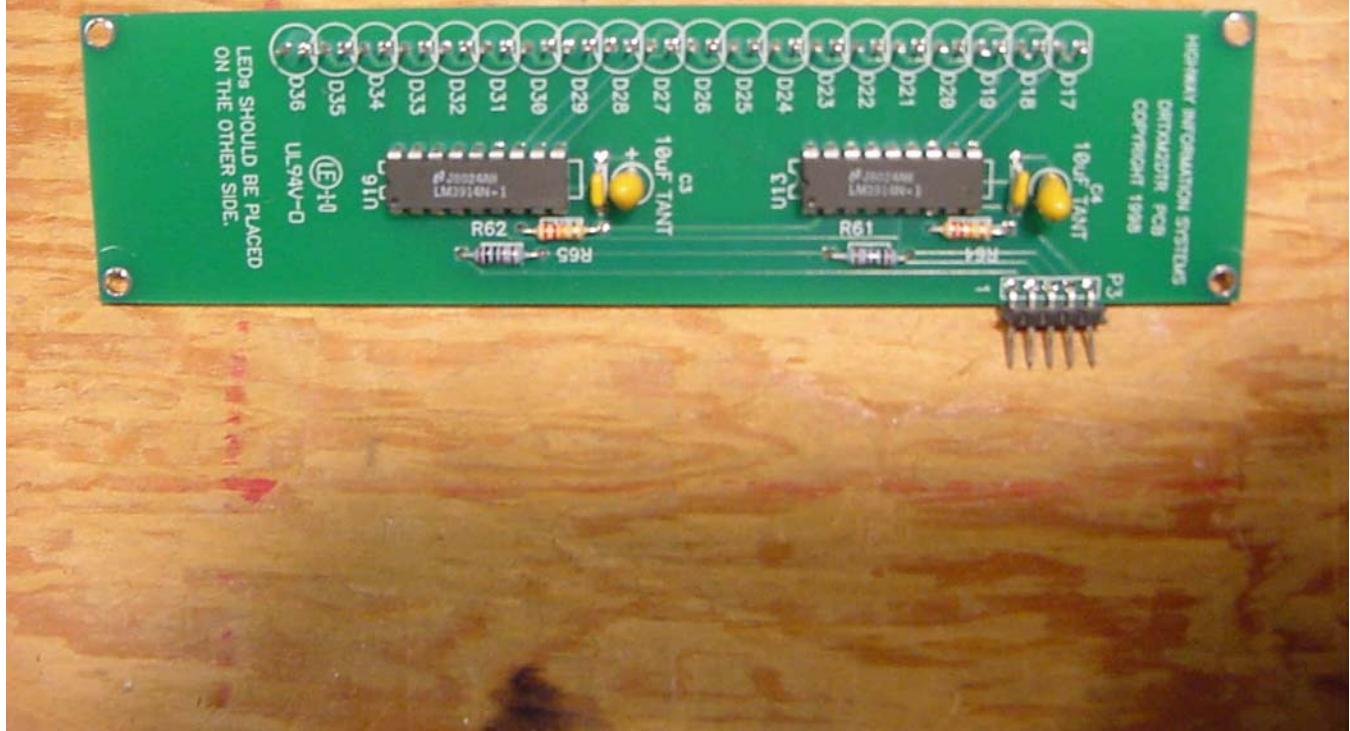
Component/LED side of the DRTXM3 circuit board
