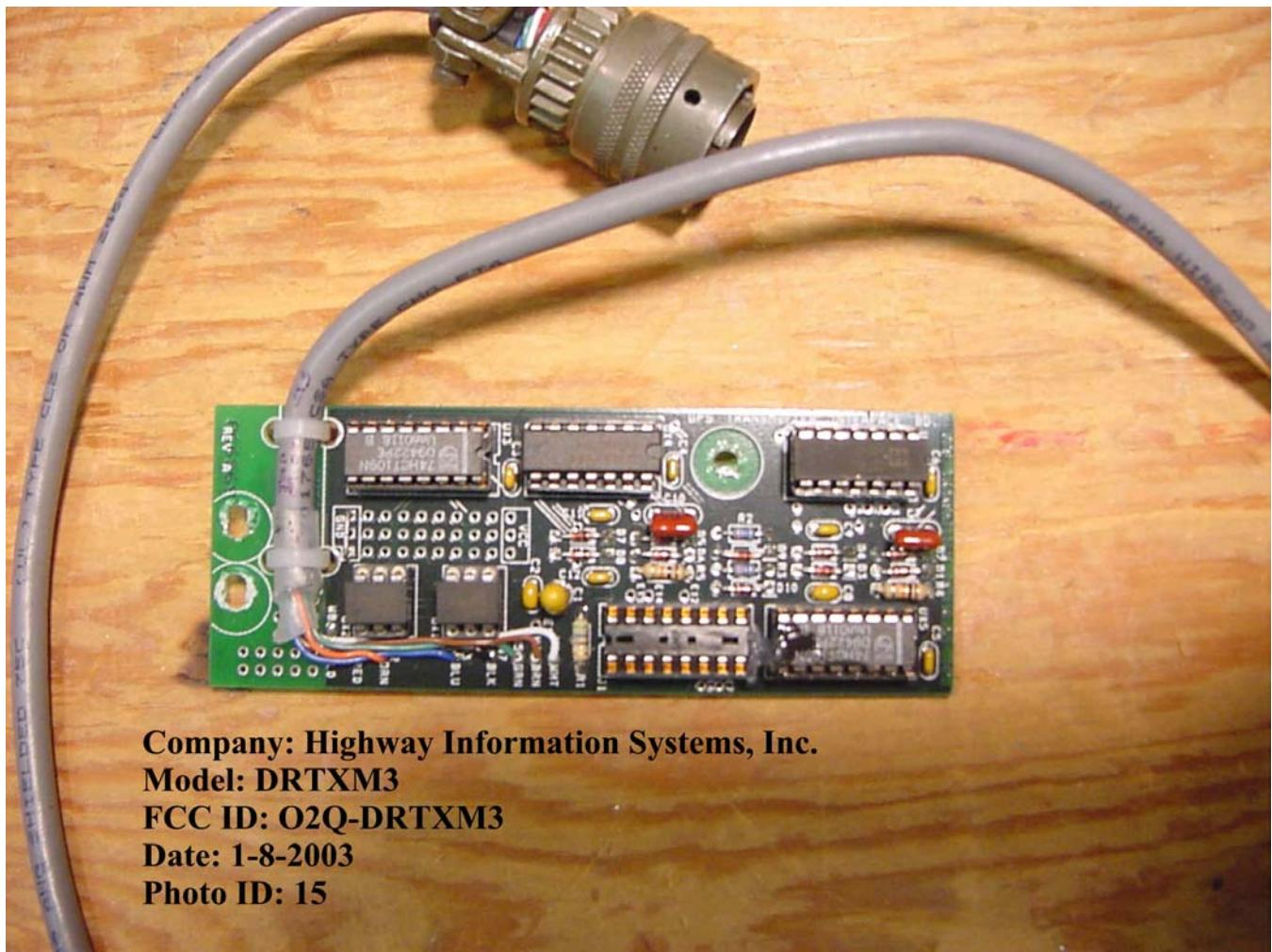
**Component side of the DRTXM3 Circuit Board
