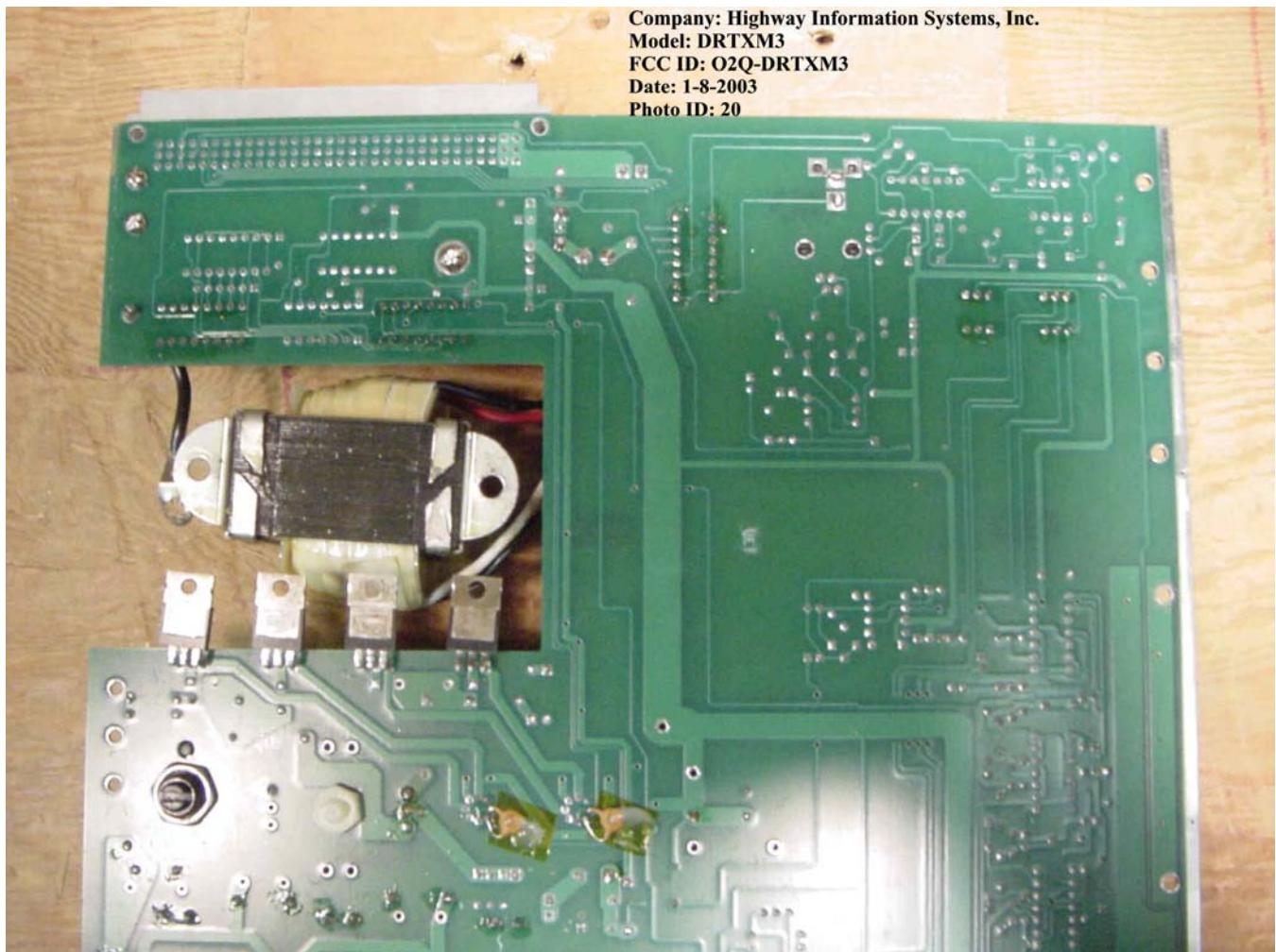
Back Half (solder side) of the DRTXM3 Circuit Board
