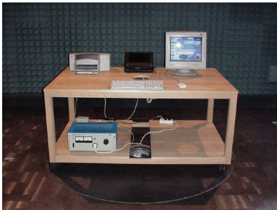
Picture 2 : RF Radiated Test set-up, front view
