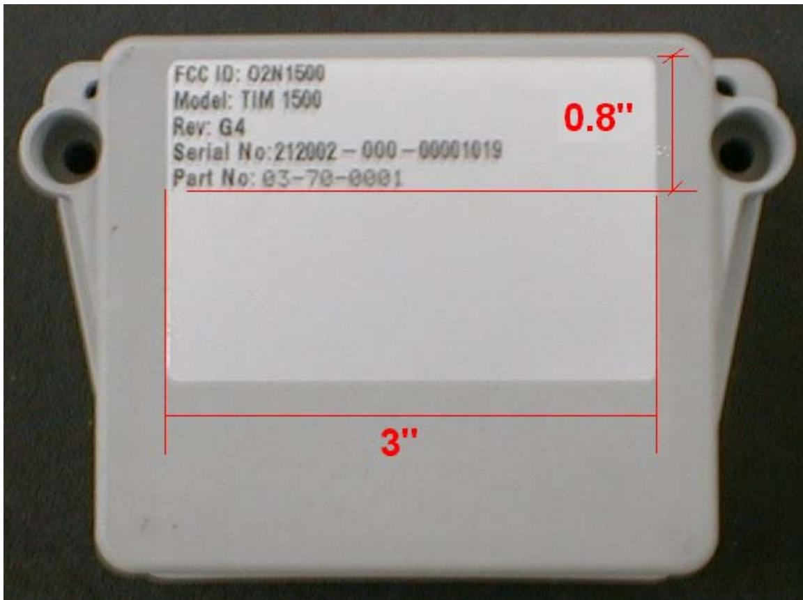
The label is made of an aluminized plastic with a high-strength adhesive backing. It is printed using nonsoluble, heat-applied ink (Brady® printing system). The label is UV- and moisture-resistant. The label should last the expected lifetime of the equipment (about 5 years) in an outdoor environment, and is not readily detachable.
