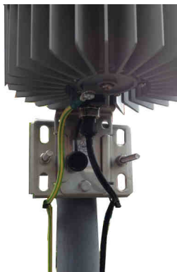
Figure 25: iR460 with Earth and Ethernet Cables Installed
