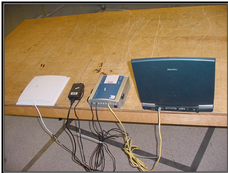
PHOTOGRAPH 11: CONDUCTED EMISSIONS TEST CONFIGURATION - PATCH ANTENNA BACK VIEW
