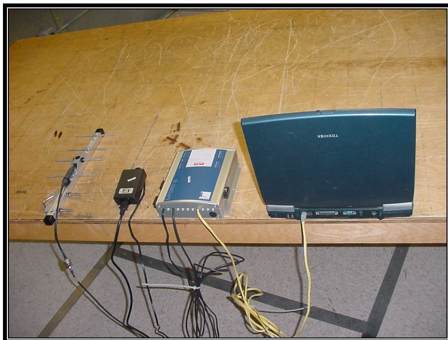
PHOTOGRAPH 13: CONDUCTED EMISSIONS TEST CONFIGURATION - YAGI ANTENNA BACK VIEW
