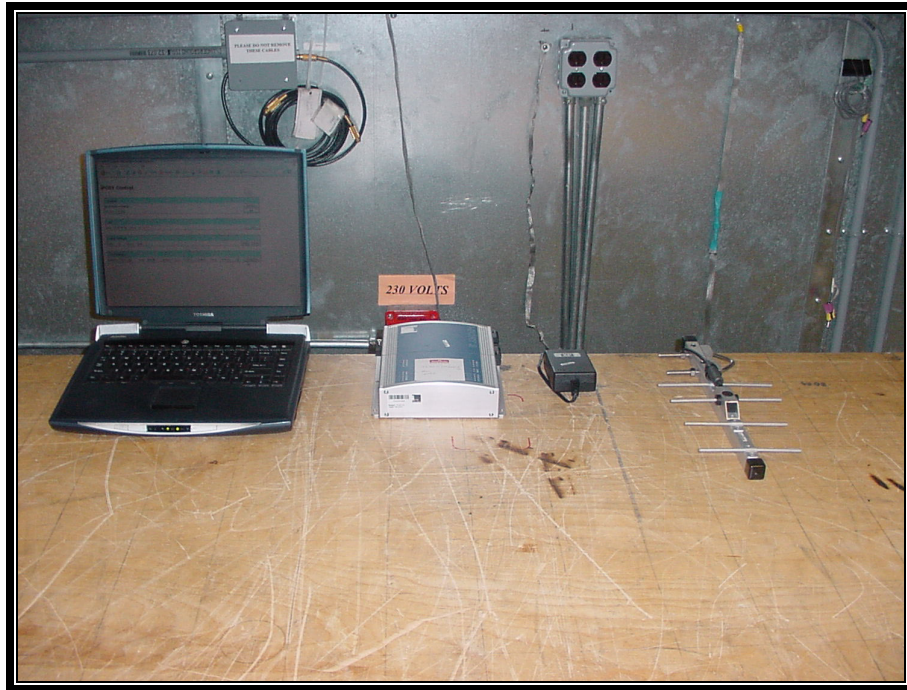
PHOTOGRAPH 12: CONDUCTED EMISSIONS TEST CONFIGURATION - YAGI ANTENNA FRONT VIEW
