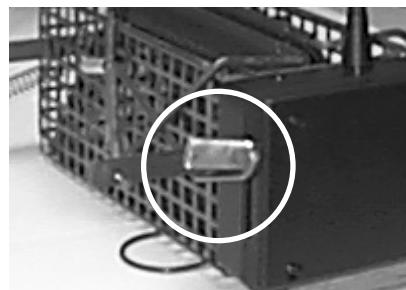
**4. Installing the hardware:** Take the bolts and lockwashers from step 1 and screw them into the ProRX from the inside of the E-Z bird launcher.
